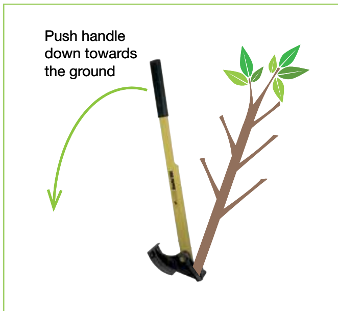
Figure 1: Using a tree popper.
