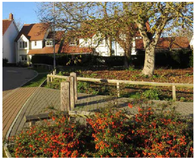
Figure 53: Appropriate material change to indicate the footpath/ cycle lane within a rural landscape, elsewhere in UK.
