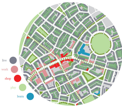
Above: This conceptual plan of a walkable neighbourhood shows how different land uses are integrated around a strong network of streets with a clearly-identifiable centre. Most homes are within a 400m or 5-minute walk of the centre, which provides for most daily needs.
