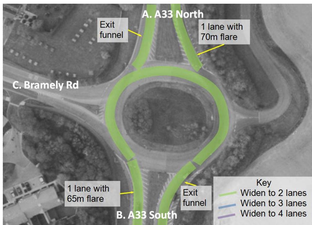
Figure 4-2 An Illustration of the Proposed Mitigation at A33 / Bramley Road Roundabout; Source: Google Maps (2013)
