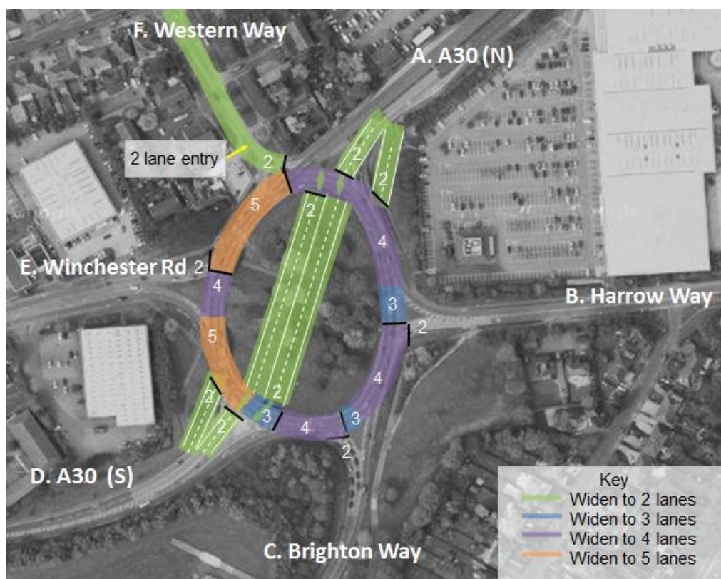
Figure 4-8 An Illustration of the Proposed Mitigation at Brighton Hill Roundabout; Source: Google Maps (2013)
