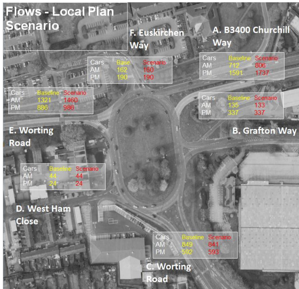
Figure 4-23 Demand at West Ham Roundabout with and without Local Plan Developments; Source: Google Maps (2013)
