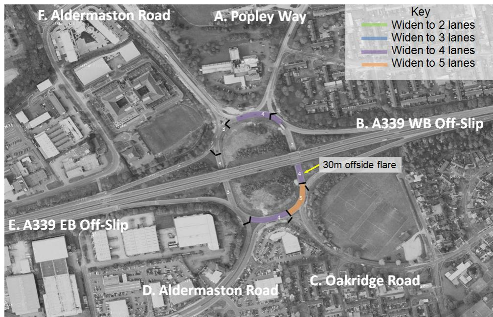
Figure 4-14 An Illustration of the Proposed Mitigation at Aldermaston Roundabout; Source: Google Maps (2013)
