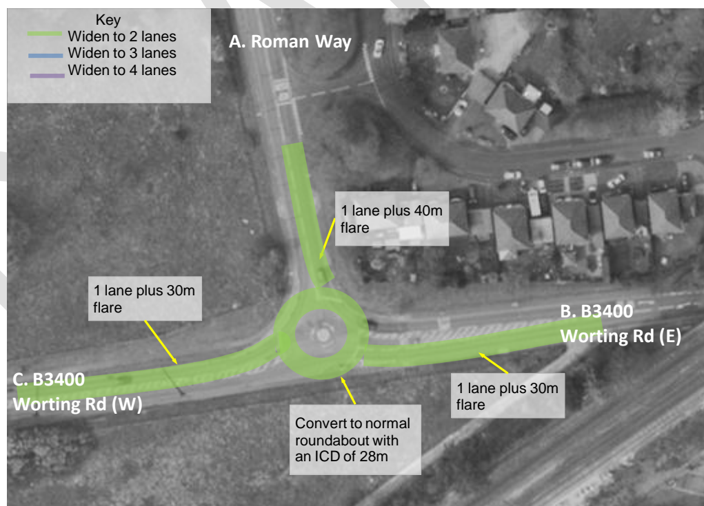
Figure 4.27 An Illustration of the Proposed Mitigation at B3400 Worting Road / Roman Way Roundabout
