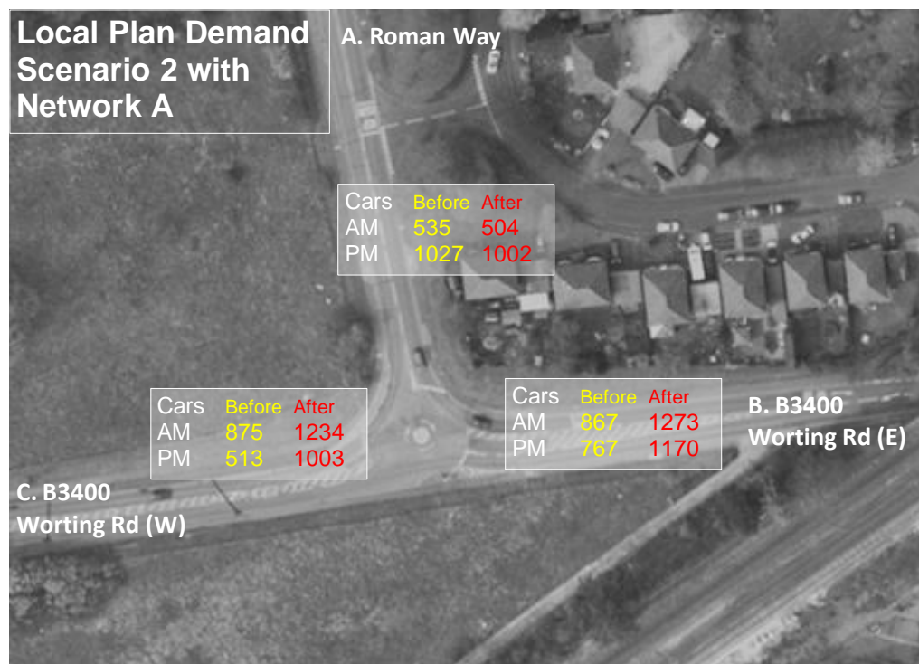
Figure 4.26 Demand at B3400 Worting Road / Roman Way Roundabout with and without Local Plan Developments
