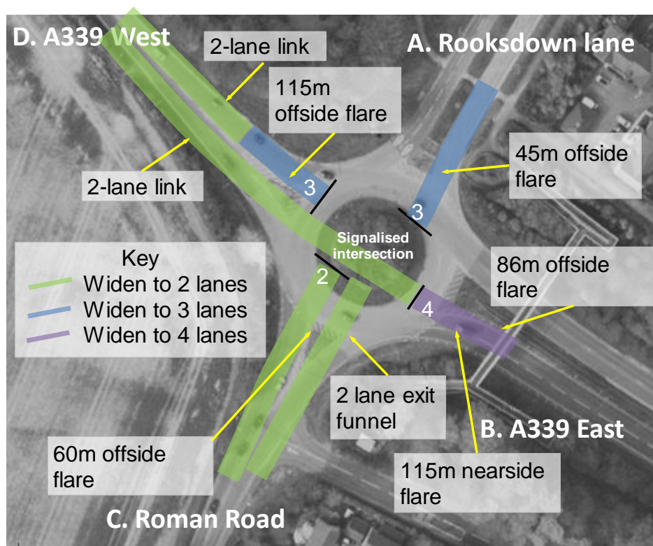
Figure 4.25 An Illustration of the Proposed Mitigation at A339 / Roman Road Junction
