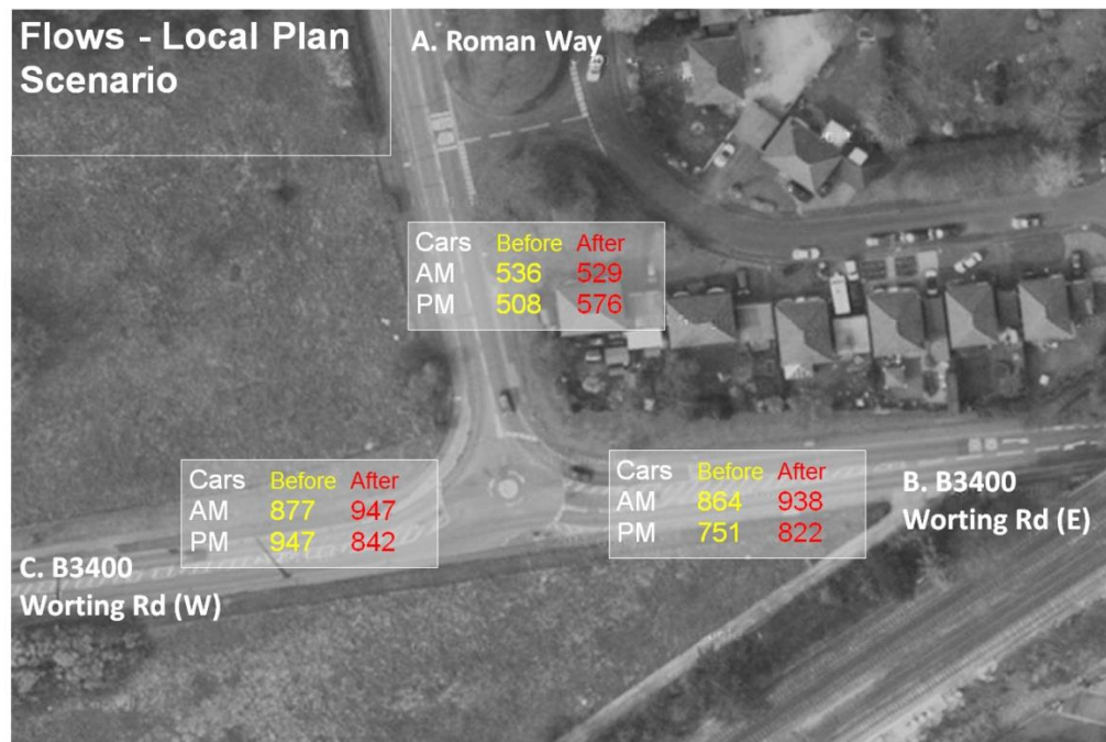
Figure 4-19 Demand at B3400 Worting Road / Roman Way Roundabout with and without Local Plan Developments; Source: Google Maps (2013)
