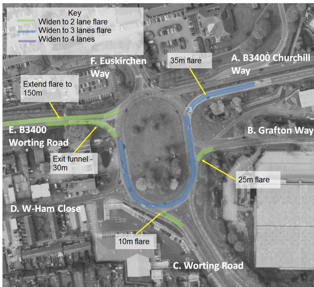
Figure 4-24 An Illustration of the Proposed Mitigation at West Ham Roundabout; Source: Google Maps (2013)
