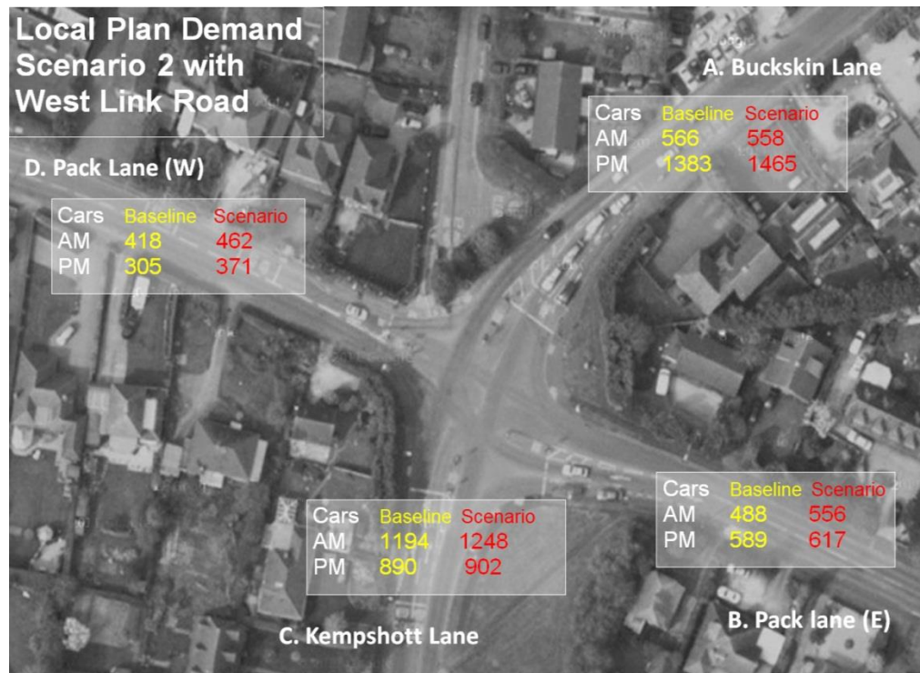
Figure 4-25 Demand at Fiveways Junction with and without Local Plan Developments; Source: Google Maps (2013)
