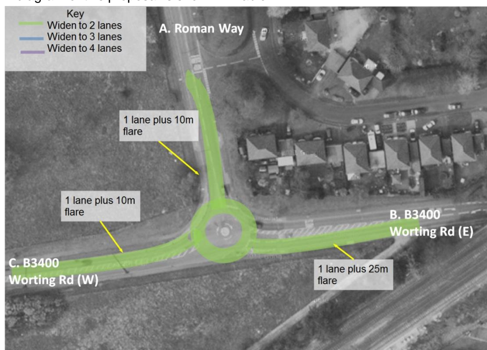
Figure 4-20 An Illustration of the Proposed Mitigation at B3400 Worting Road / Roman Way Roundabout; Source: Google Maps (2013)
