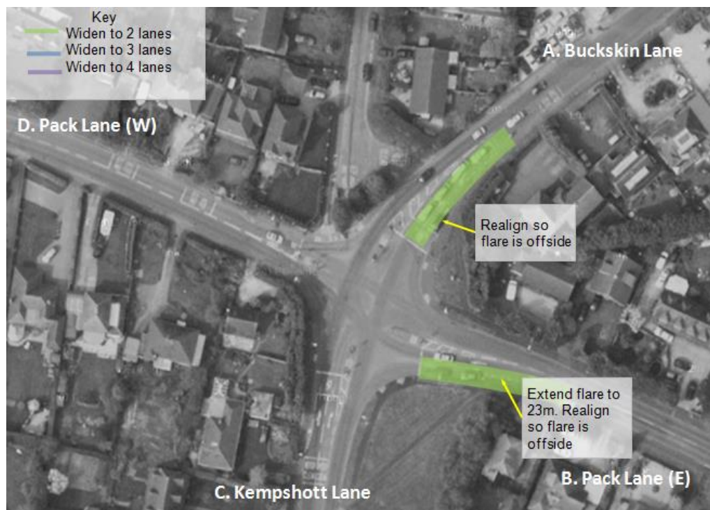
Figure 4-26 An Illustration of the Proposed Mitigation at Fiveways Junction; Source: Google Maps (2013)
