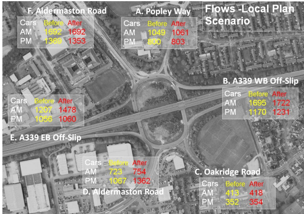
Figure 4-13 Demand at Aldermaston Roundabout with and without Local Plan Developments; Source: Google Maps (2013)
