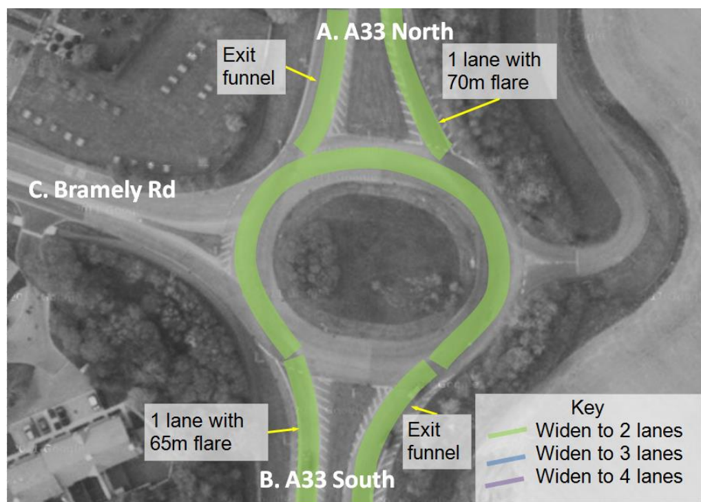
Figure 4-2 An Illustration of the Proposed Mitigation at A33 / Bramley Road Roundabout; Source: Google Maps (2013)
