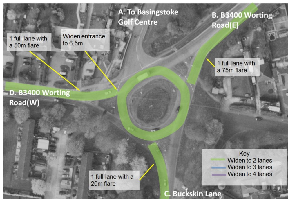
Figure 4-22 An Illustration of the Proposed Mitigation at Worthing Road Roundabout; Source: Google Maps (2013)
