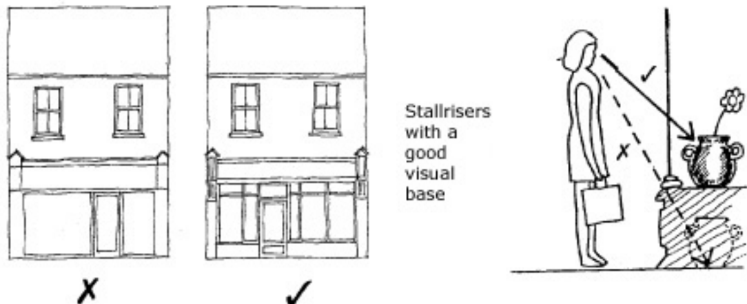
Figure E5: Examples of good and bad practice in the design of the base of a shopfront, illustrating the importance of stallrisers.
