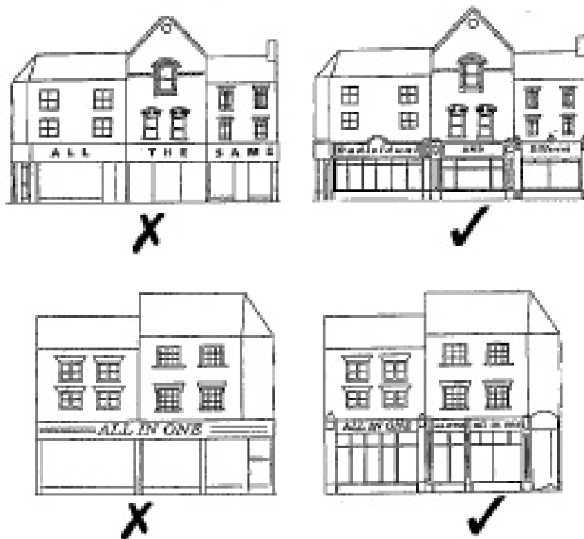
Figure E4: Examples of good and bad practice in the design of fascias where two or more buildings are in the same business use.
