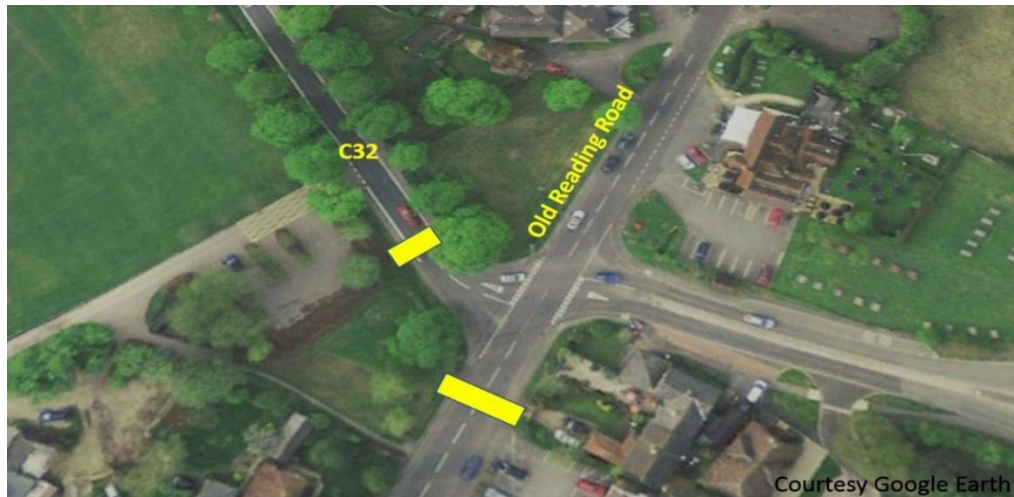
Figure 4-1 Two proposed sites for pedestrian crossings at junction C32 with Old Reading Road
