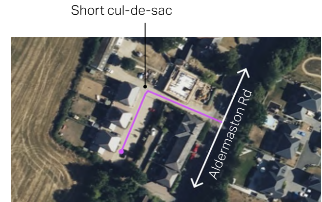
Figure 94: Aerial image of Lavers Lea off Aldermaston Road. This layout of a short cul-de-sac behind linear development with an access road between the front of properties and the back of existing properties is a more acceptable development layout and could be appropriate in some areas of Sherborne St John.
